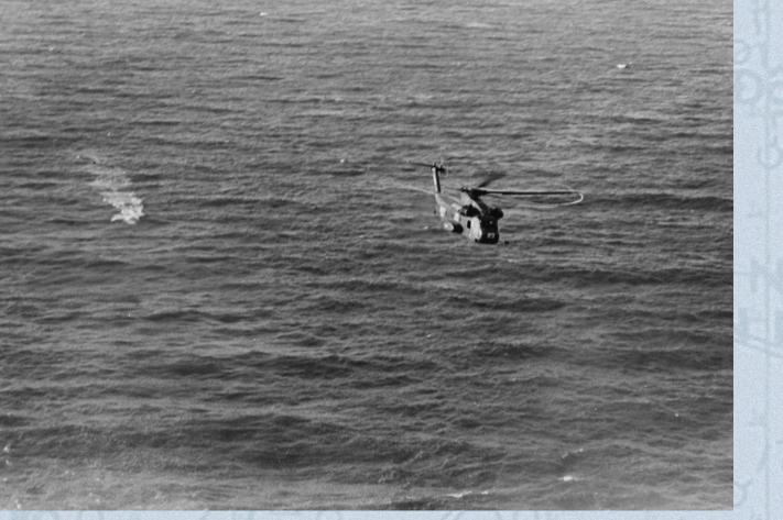
Operation END SWEEP. A CH-53A Sea Stallion tows a Magnetic Orange Pipe (MOP) to detect mines for clearing Haiphong Harbor. To reduce collateral damage after U.S. demands were met in peace negotiations, U.S. Navy ships and aircraft cleared Vietnamese waters of mines. (U.S. Navy / National Archives)
